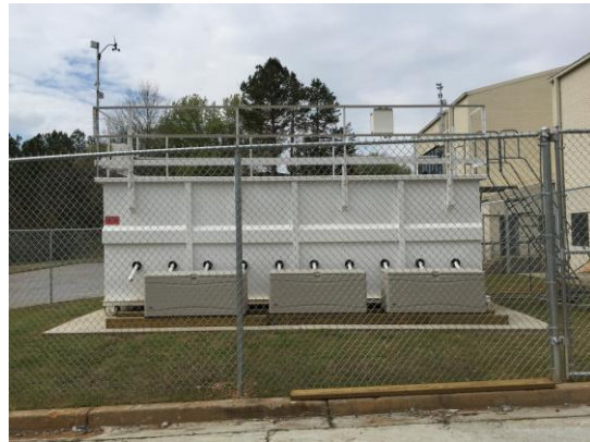
Figure 6.2: Lysimeter test bed located behind CETL.
