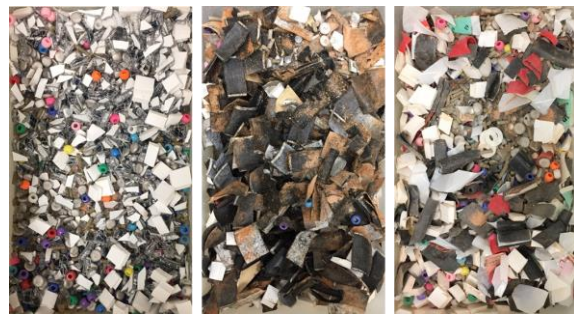
Figure 7.3: E-wastes (left to right: c-Si module, NiMH battery, Li-ion battery) mixed with MSW components and soil before packing in columns.
