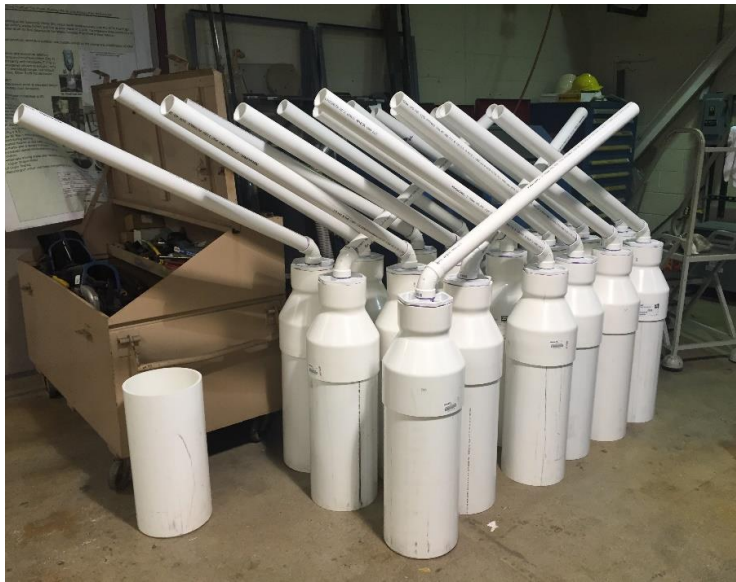
Figure 6.6: Outer casings for the lysimeters prior to installation in the test bed.
