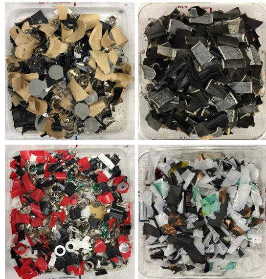
Figure 7.1: Disassembled and shredded NiMH outer casings (top left), Li-ion outer casings (bottom left), NiMH electrodes (top right), and Li-ion electrodes (bottom right).
