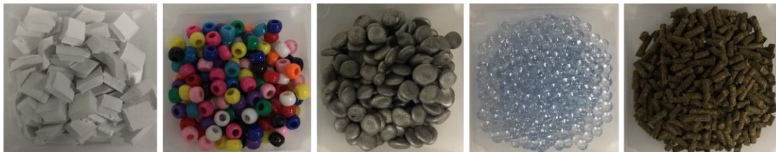
Figure 7.2: MSW components: from left to right: paper, plastic, metal, glass, and food.
