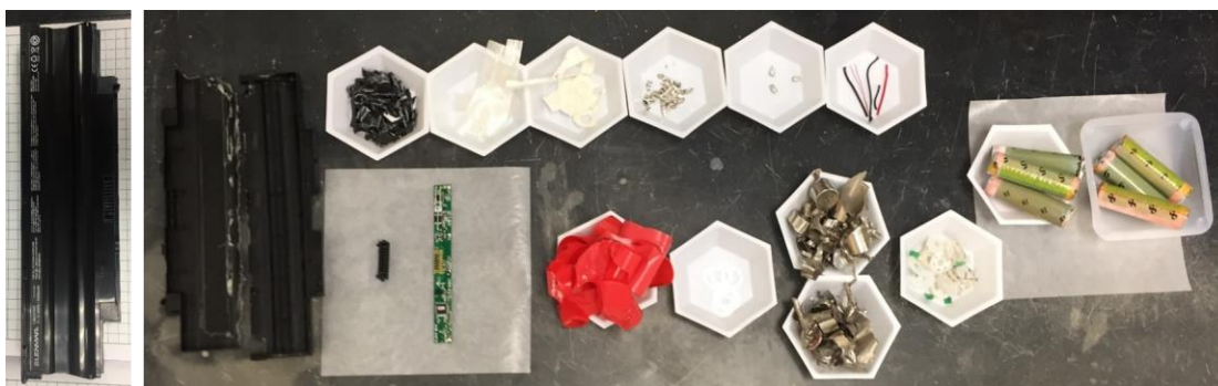
Figure 8.3: Images of the Li-ion laptop battery, including disassembled components.
