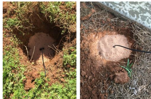
Figure D.1: Placement of Decagon 5TE sensors in the ground near the test bed.
