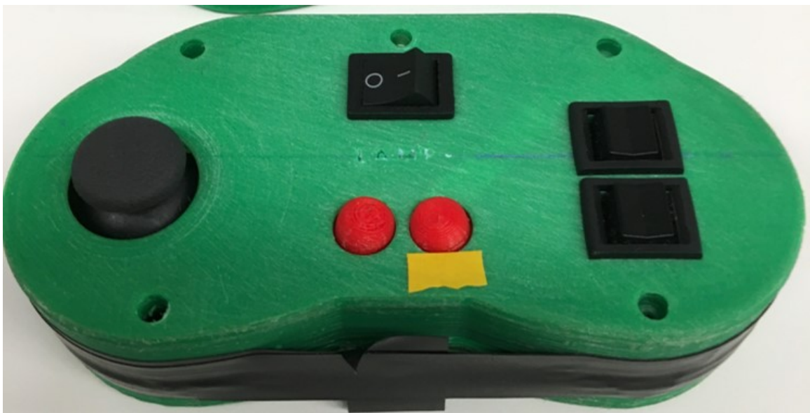
Figure 2.5: Tele-operation method of the h+lamp hardware using custom-built controller and Bluetooth.
