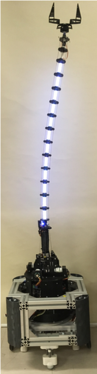
Figure 3.1: Third generation continuum robotic mobile lamp (CuRLE) with internal LED strip lit.
