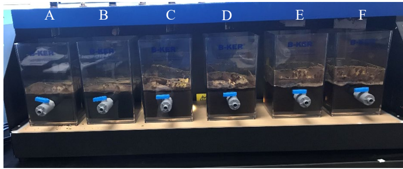
Figure B-2: Jar experiment after rapid mixing for pH 8.2 (top), pH 5.5 (middle), and pH 6.5 (bottom) samples with 1 g/L (A, B), 5 g/L (C, D), and 10 g/L (E, F) FeCl 3 dosages.
