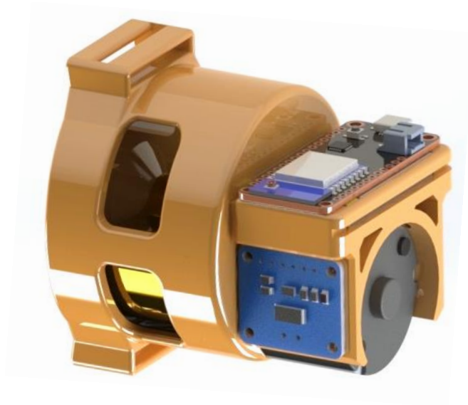
Figure C-2. CAD rendering showing assembled energy harvester
