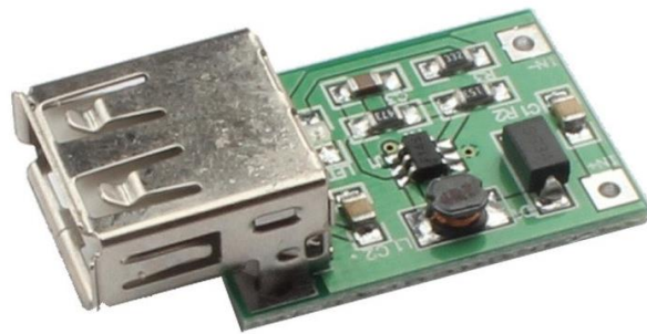
Figure C-8. Photograph of the 5VDC Boost converter
