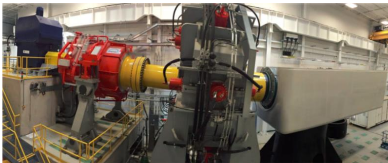
Figure 3.2: Clemson University 7.5-MW test bench with Nacelle enclosing a multi-MW drivetrain (photo credit: Konstantin Bulgakov).
