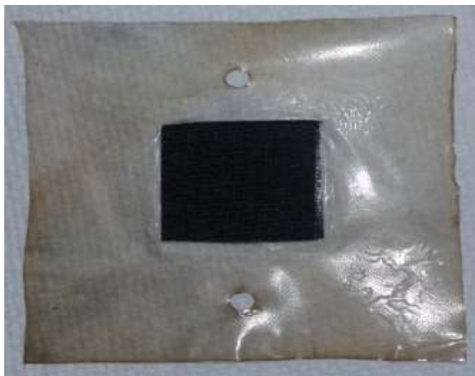
Figure 2.3. Photomicrograph of the large-scale MEA fabricated for a conventional fuel cell station. The MEA has been used on a Scribner model 850C fuel cell test station. See detailed description of the MEA dimension in the text.
