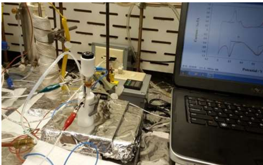
Figure 7.23. Photograph of small liquid electrolyte alkaline PTFE cell.
