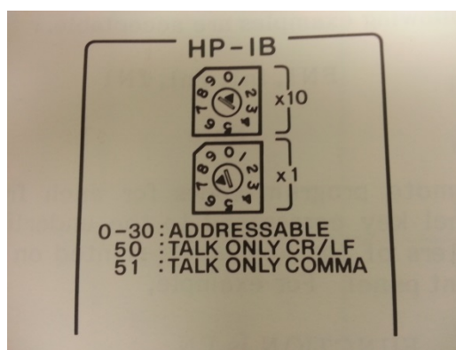
Figure 2: HPIB settings for the HP 4280A (located on the back). The dials should be adjusted to address ‘51: Talk Only Comma’. (Note: The address shown in the image above is 17).
