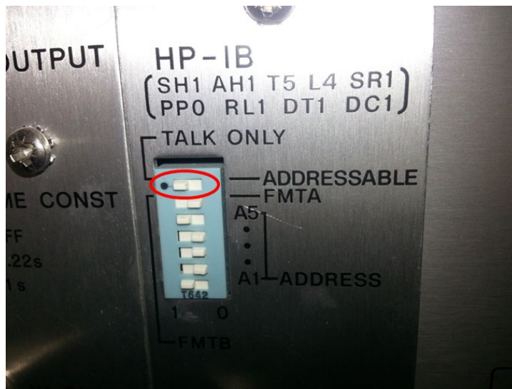
Figure 4: HPIB setting for the HP 4140B (located on the back). The switch circled in red should be positioned to the left; 'talk only' (color version on computer).
