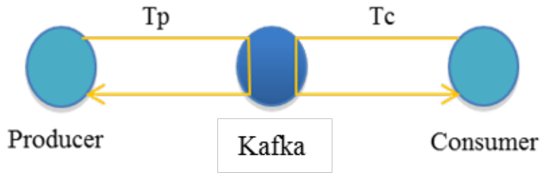
Figure 3.5: Breakdown of an end-to-end latency of a message delivery procedure using the developed message delivery system.
