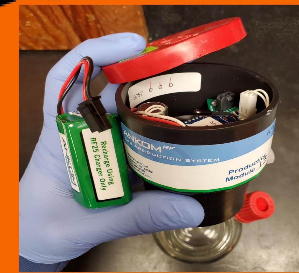
Figure 1. Gas production module has a sensor sending signals to the computer
