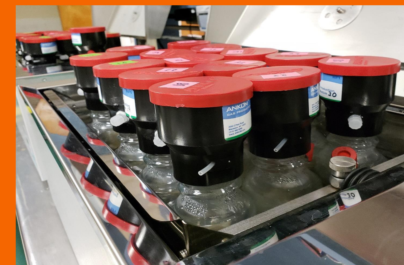
Figure 2. Water baths and shakers to incubate the modules in 39°C for 24 h
