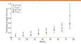
Adsorption isotherms indicates the surface affinity of water. Each data point is composed of eight isotherms at different temperatures ranging from 5-23°C. The increase of thickness of water is shown as a function of increasing RH.<sup>2</sup>
