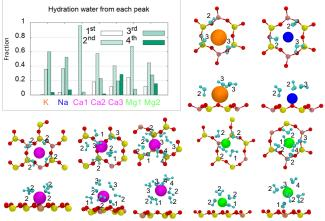
Ion hydration shell composition and snapshots. Labels on the snapshots indicate the water peak in density profile. Yellow, red, pink are mica surface atoms. Orange: K, blue: Na, magenta: Ca, green: Mg.
