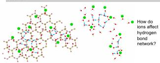
Hydrogen bond network in Mg2+-mica. Blue arrows indicate hydrogen bond between water molecules
