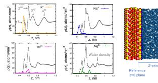
Ion density and water density on mica surfaces in z-direction at 300K. Grev curves are water density plots. A snapshot of simulation box is given on the right.
