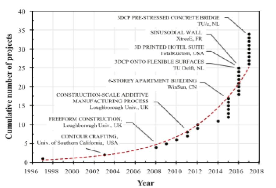
Figure 1: The rise in large-scale additive manufacturing for construction applications since the concept inception in 1997.
