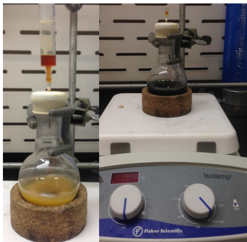
Figure D.2 Chemical polymerization of PEDOT basic set-up
