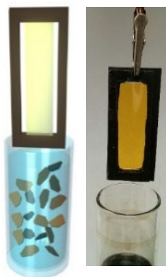
Figure 5.4: Deposition of a monolayer of GO-P2 on flexible polymeric substrate.
