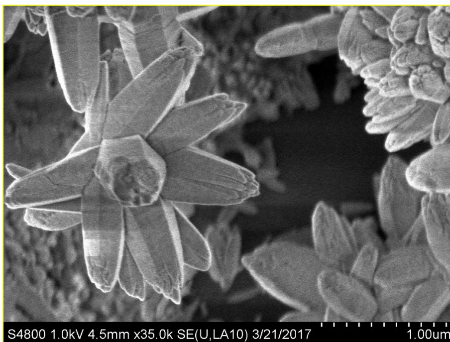
Figure A35: ZnO nanorods grown by hydrothermal method on rGO-P1 mono- and bilayer films.
