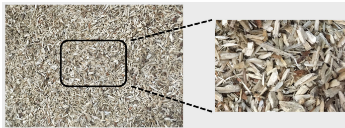
Figure 5.1: Loblolly pine forest residues after being hammermilled with a 25 mm screen.
