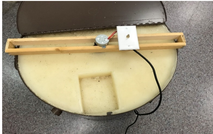
Figure 4.16. Neutron howitzer with motor assembly attached to rotate the source port.
