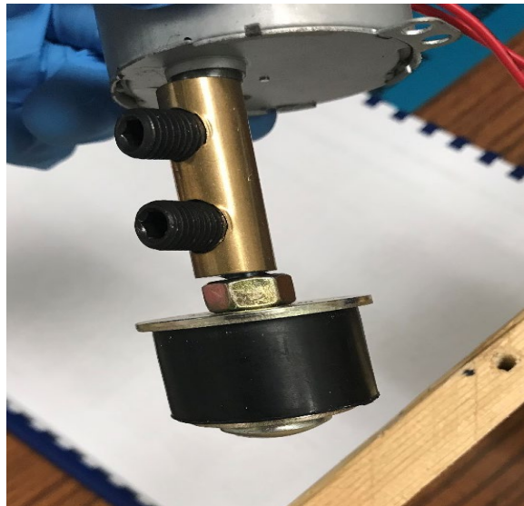
Figure 4.17. Expansion plug attached to motor shaft.
