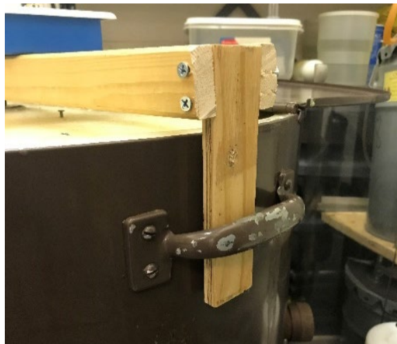
Figure 4.19. Motor structure anchored into howitzer handles.
