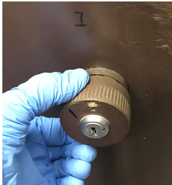
Figure 4.10. Port cap added to port 1.
