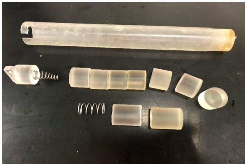
Figure 4.2. Sleeves, spacers, springs and end caps used in the sleeve assembly.
