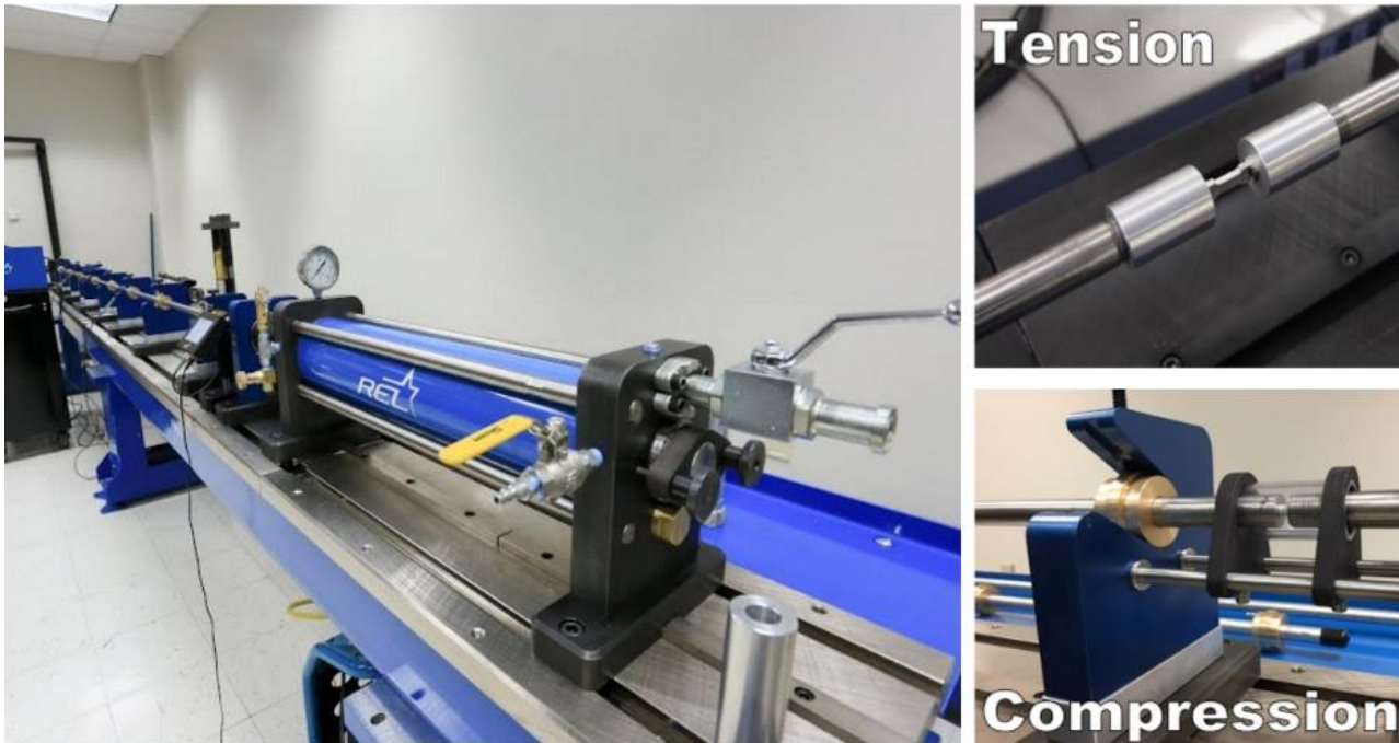
Figure 11: Split Hopkinson pressure bar (Provided by Joe Indeck from Dr. Hazeli's research group (MMEE) University of Alabama in Huntsville.)
