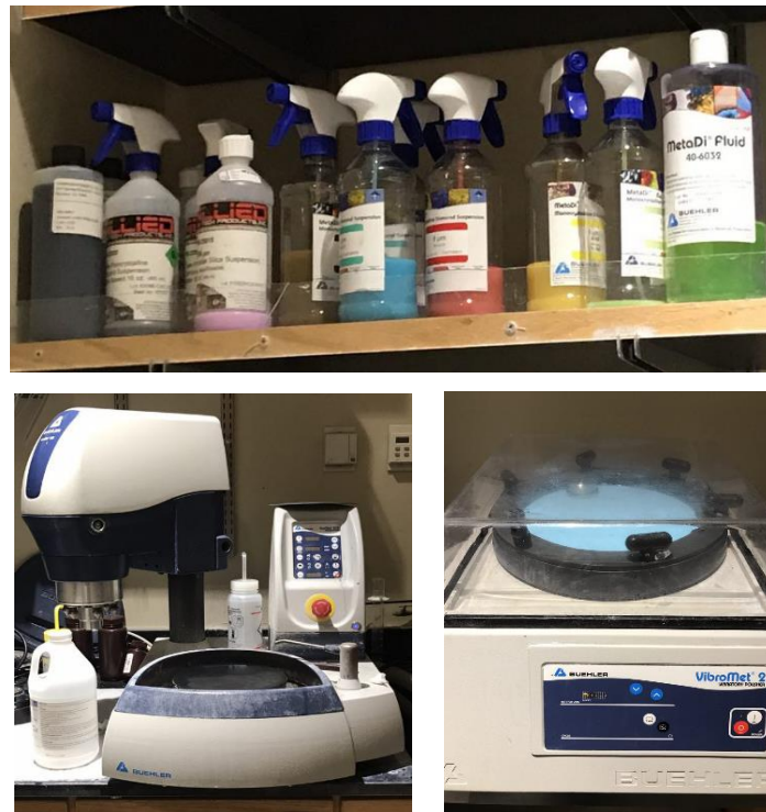
Figure 12: Diamond pastes, polisher and vibro-polisher used to prepare the samples for EBSD.
