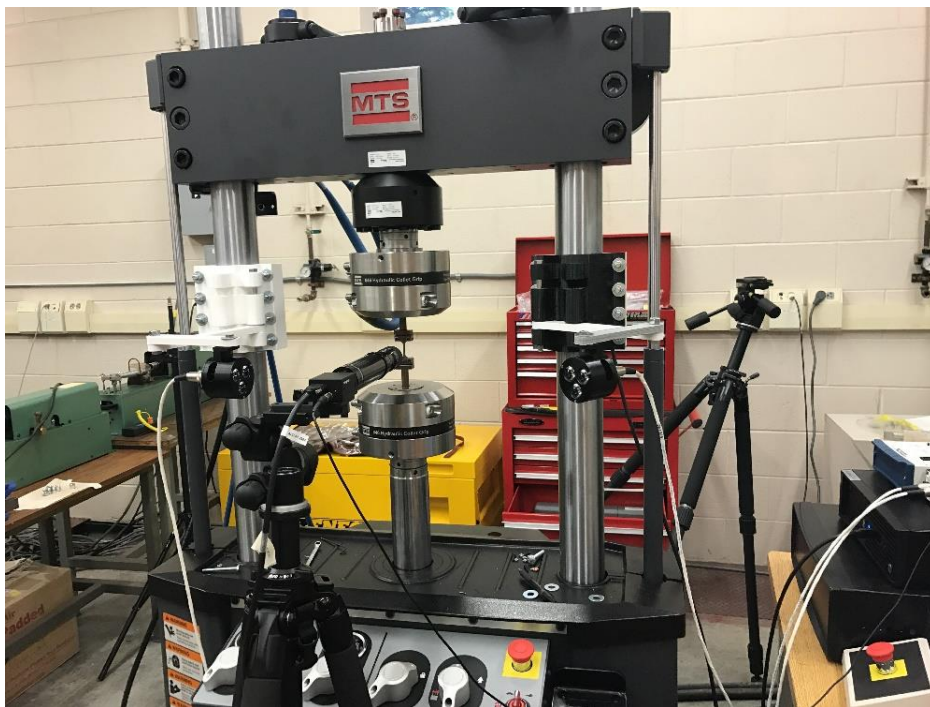
Figure 5: Camera set-up to use DIC for the tensile experiment
