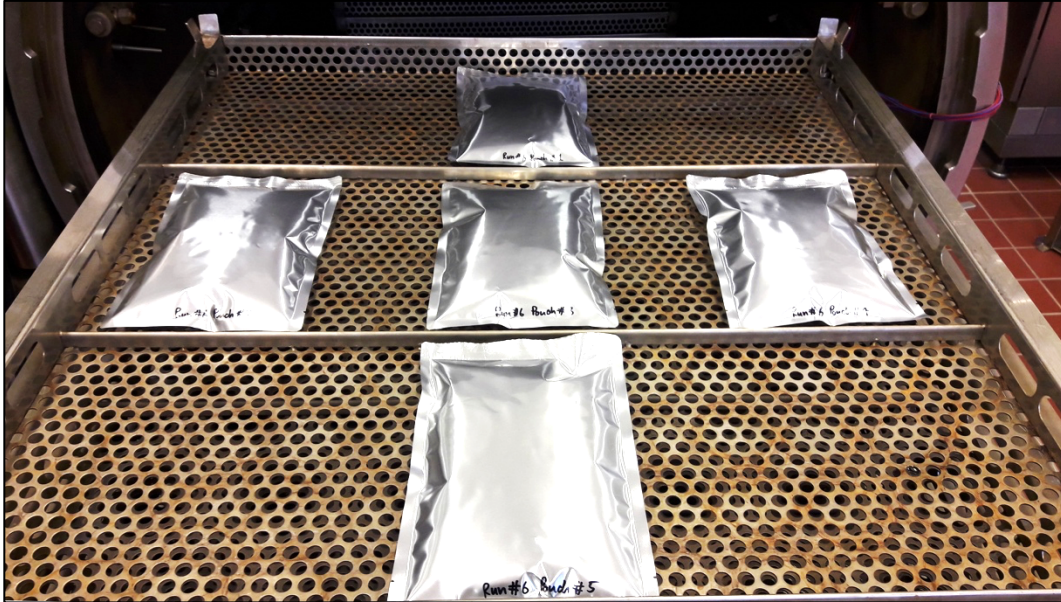
Figure 3.1. Pouch arrangement on the retort rack.
