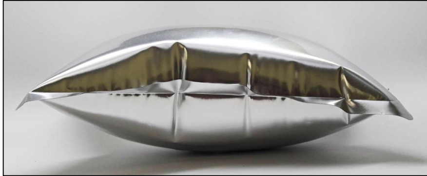
Figure 4.10. Internally pressurized pouch.
