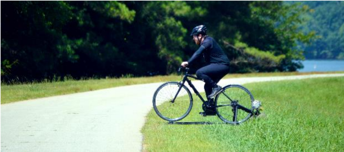
Figure 4.3 A magnified daytime photograph of the nighttime setup. During testing the bicyclist displayed one of the six Light Placement levels from Table 2.1. The test bicyclist wore all-black apparel (including shoes) that contained no reflective elements.
