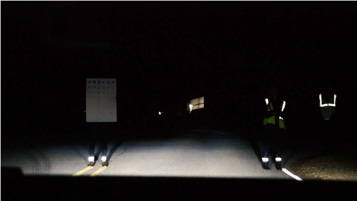
Figure 2.5 A still image taken from the recording of the camera calibration session, which took place at Hugo Drive. Three researchers – one of which was holding a Pelli-Robson contrast sensitivity chart – stood in front of the test vehicle while experimenters in the vehicle calibrated the camera’s video settings. Experimenters in the test vehicle adjusted the camera’s settings until the contrast and color characteristics of the video matched what could be seen by the eye.
