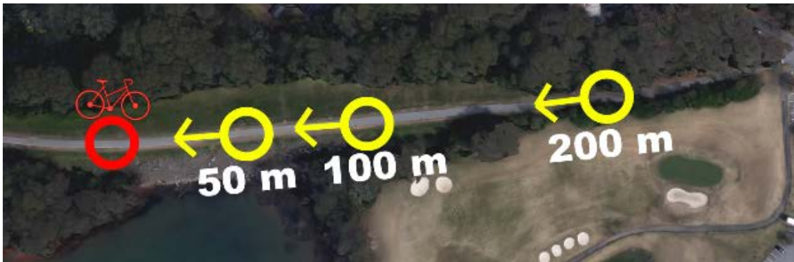
Figure 4.2 A satellite image of the service road used to collect data in Experiment 2. The red circle indicates the position of the test bicyclist at the easternmost end of the 200 m straight section. The yellow circles indicate the positions of the stationary test vehicle at the marked 50 m, 100 m, and 200 m observation points. The yellow arrows indicate participants' viewing direction (west), looking towards the stationary test bicyclist.
