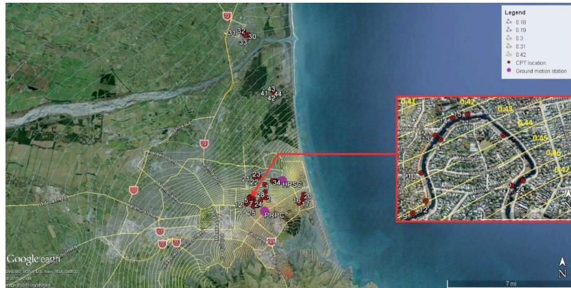
Figure 3.1: Contour map of the computed median of conditional PGAs for the 22 February 2011 earthquake (Bradly & Hughes 2012). Inset is a zoom-in view of the studied area showing contours of PGAs and locations of CPT data.
