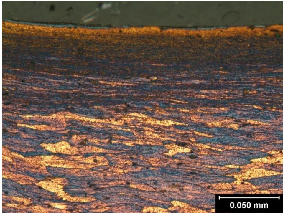
Figure 9-37: Etched material near the screw-workpiece interface – sample 5 bottom
