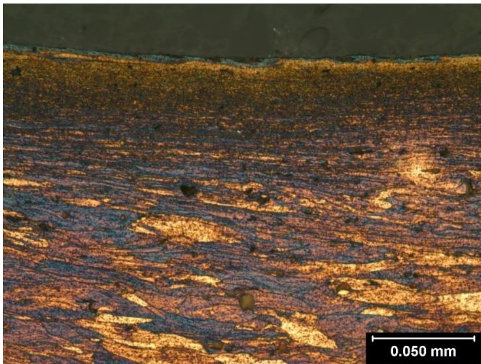
Figure 9-46: Etched material near the screw-workpiece interface – sample 6 bottom
