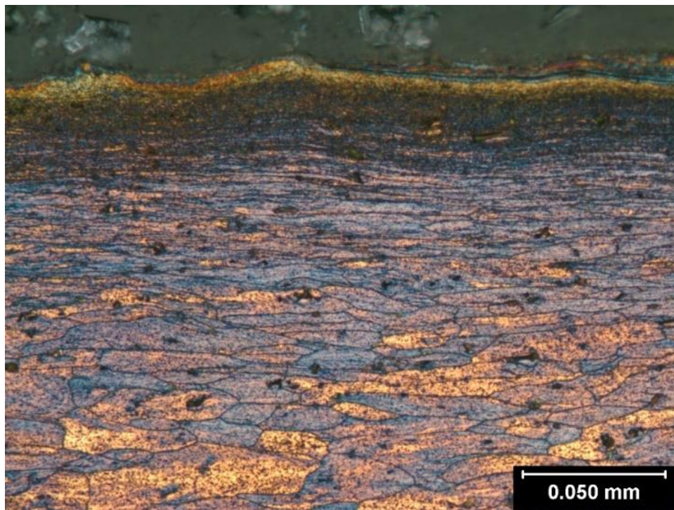
Figure 9-40: Etched material near the screw-workpiece interface – sample 6 top
