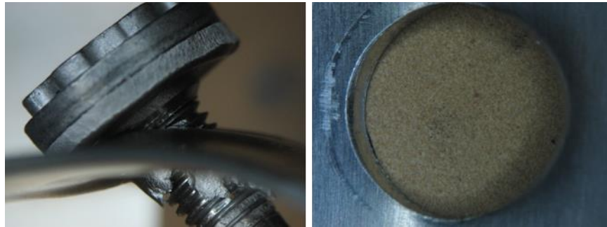
Figure 3-14: Fractured static lap shear sample
