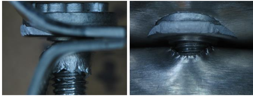
Figure 3-13: Fractured static coach-peel sample
