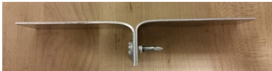
Figure 3–12: Coach-peel sample configuration
