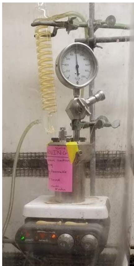
Figure 4.9: Parr pressurized vessel utilized for high-pressure hydrogenation at room temperature.
