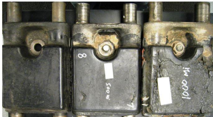
Figure 1.2 Progression of Backer Pad Deterioration due to Hysteretic Heat Loss [5]
