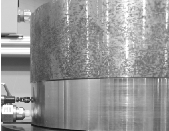
FIGURE 4. LARGE MASS PART (M = 20.0 KG), SHOWING UNFINISHED (UPPER) AND FINISHED (LOWER) SURFACES.
