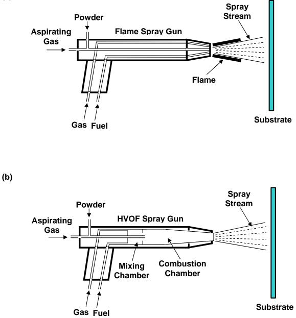
Figure 5. A schematic of the: (a) Flame; (b) High-velocity Oxygen Fuel (HVOF) and (c) Plasma-arc Thermal Spray process.
