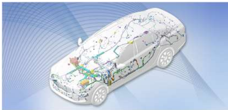
Fig. 3.1. Wire harnesses in an automobile.
