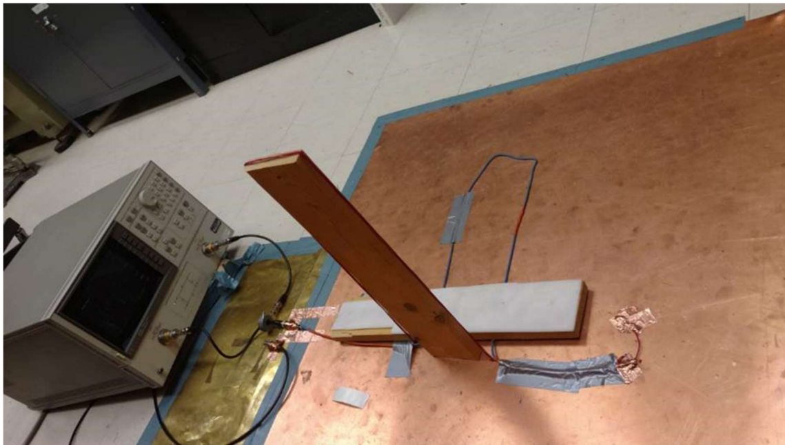
Fig. 3.9. Test set-up for the detached twin wire pair from the ground wire
