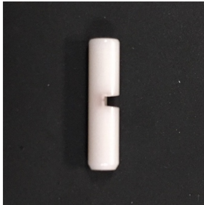
Figure 5.5 Ceramic cutting test with ps laser micromachining system
