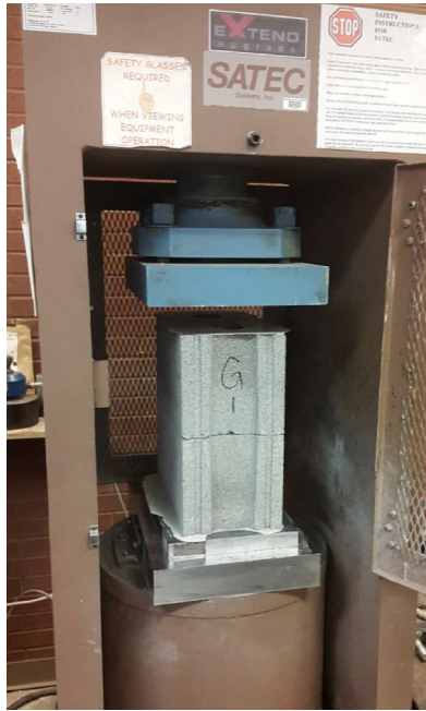
Fig. 3-4. Experimental setup for prism masonry test.
