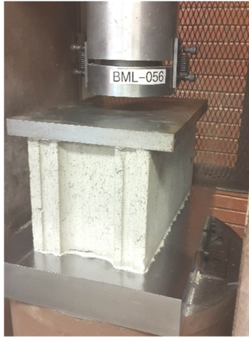
Fig. 4-6. Experimental setup of the CMU test.
