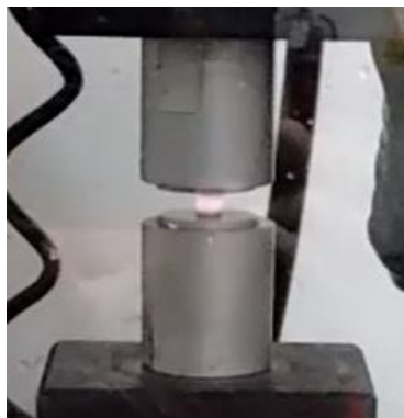
Figure 9-14: WC with a current density of 50A/mm 2 , note the color change due to heat
