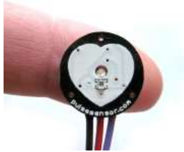
Figure 9. Pulse Sensor Amped conveying the emitter, detector, and size
