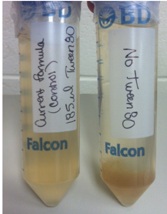
Figure 3.5. Coating formula stability after 6 weeks. (Left: Control coating formula containing Tween® 80; Right: Treatment formula that does not containing Tween® 80)
