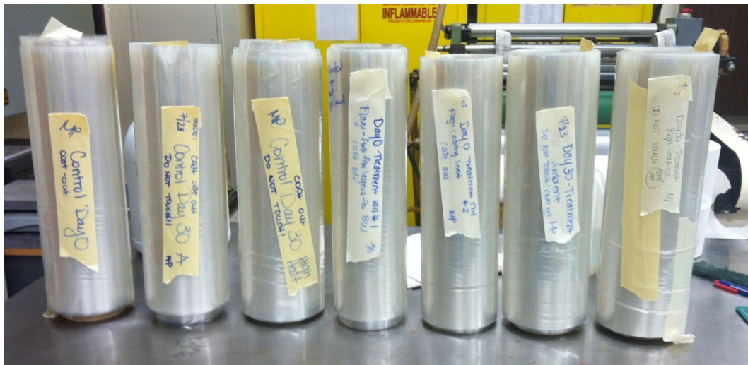
Figure 4.7. Rolls of coated material produced during gravure coating trials.
