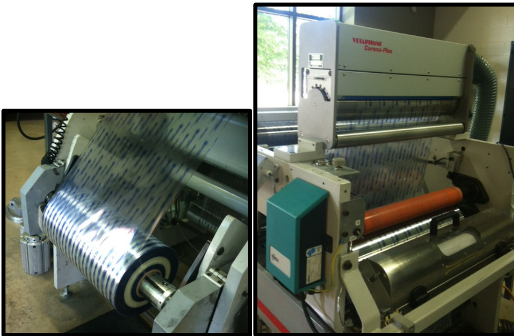
Figure 4.17. Uncoated web at the unwind station (left) moving into the corona treater. (right)
