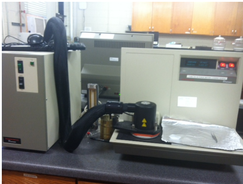
Figure 3.1. DSC 2920 modulated DSC used for determining polyvinyl alcohol resin grade and plasticizer combination.
