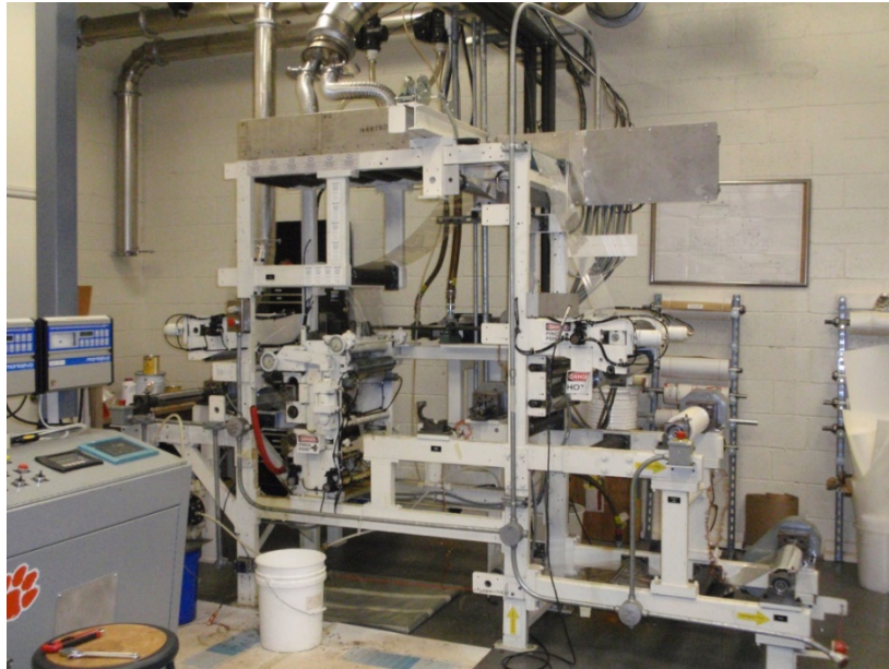
Figure 4.5. Solvent-based coater/laminator in DuPont laboratory Clemson University.
