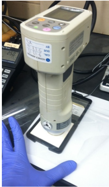
Figure 4.10. Haze testing with colorimeter.
