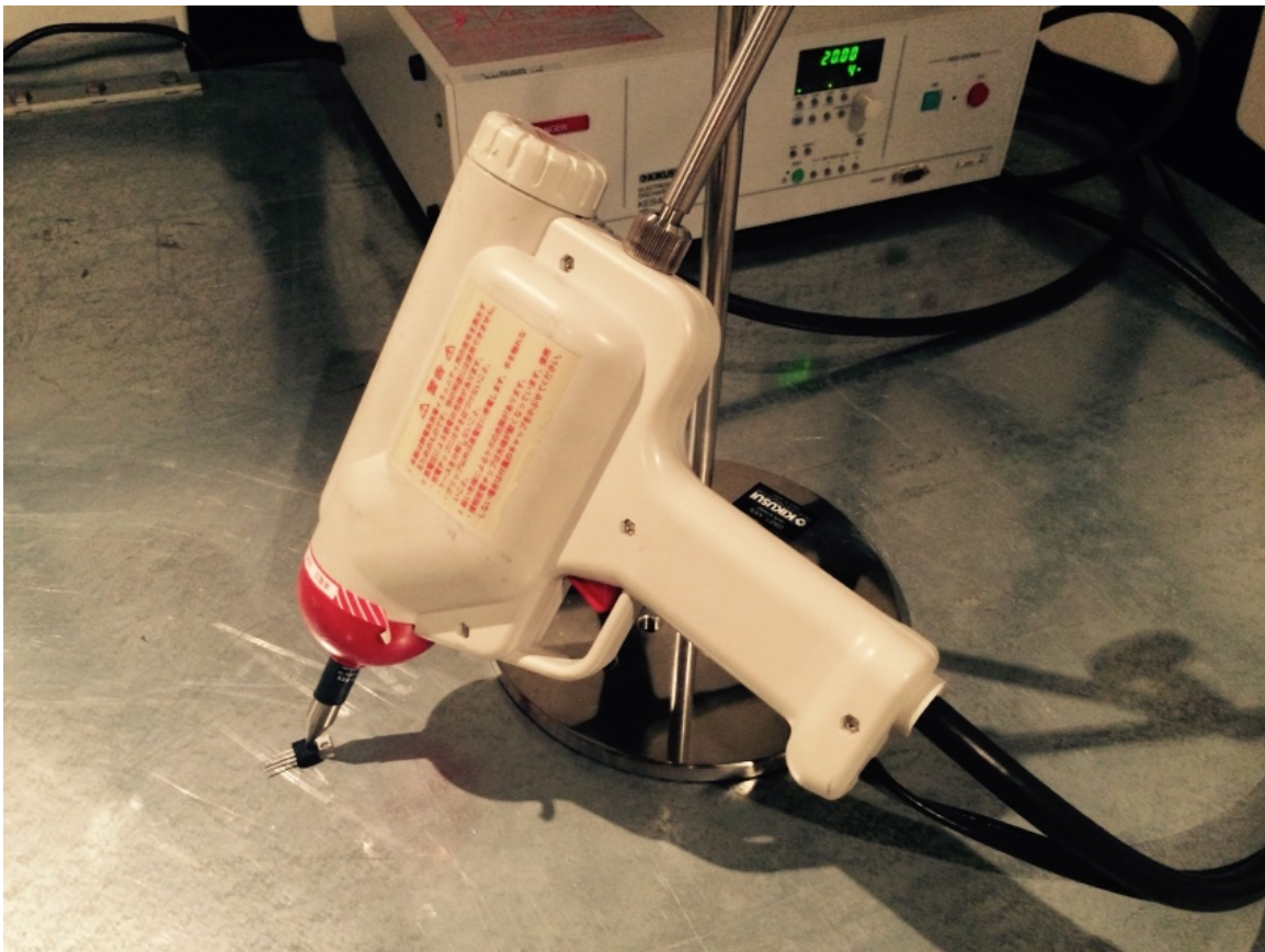
Fig. 1.9. Setup used to perform ESD degradation of MOSFET transistors.
