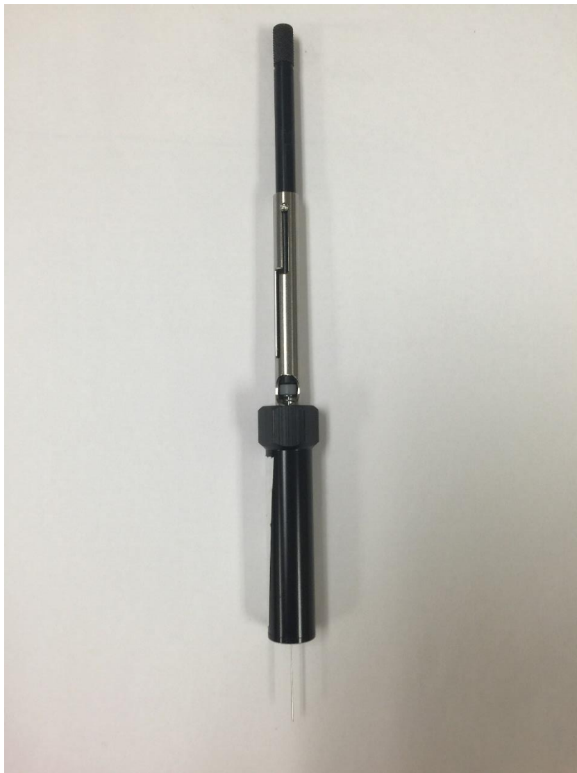
Figure 1. 3 The Device for SPME
