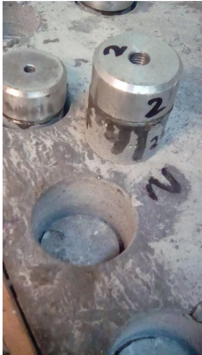
Figure 65: Failure of Test Specimen at the UHPC to Precast Interface
