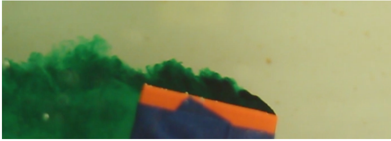
Figure 2.11: Dye injection photograph of flow around square cylinder at 13^\circ incidence. Re = 4900 .
