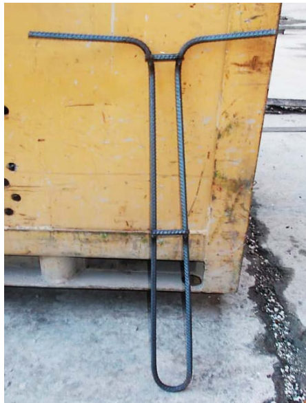
Figure 14. Custom #3 stirrup used as transverse reinforcement
