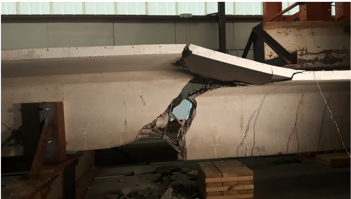
Figure 36. Flexure-shear failure in the specimen N1
