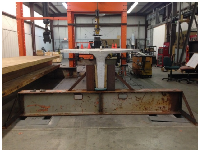
Figure 19: Specimen braced by “saddle” at each support
