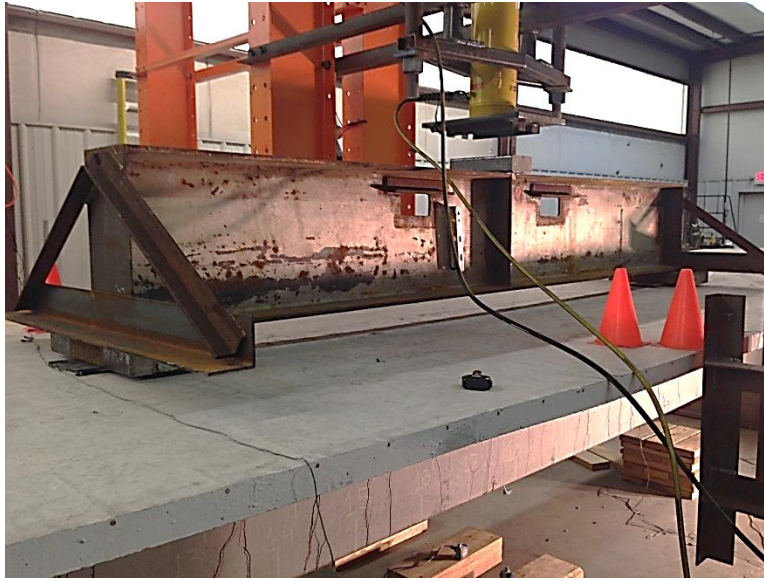
Figure 20. I-beam used for spreading load from jack to specimen
