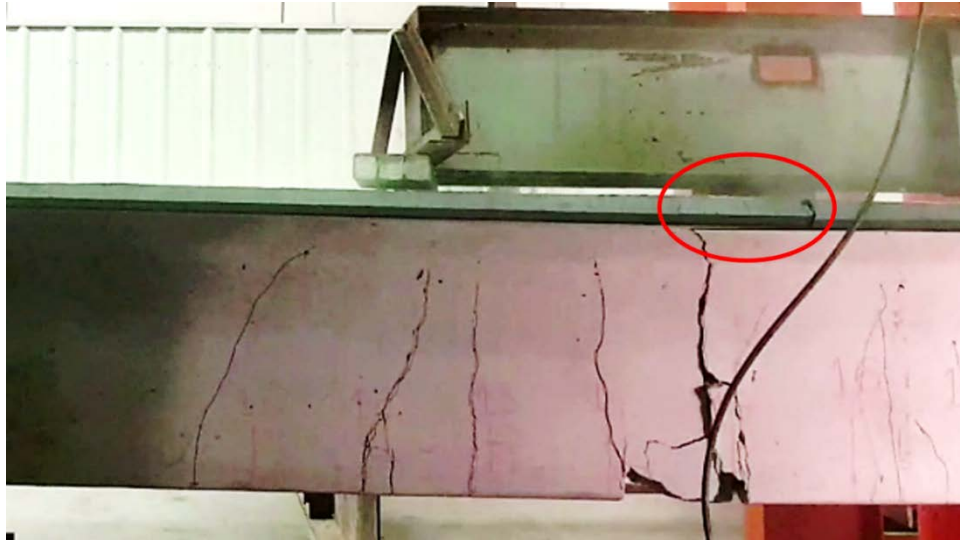
Figure 37. Compression zone shear failure in the specimen N2
