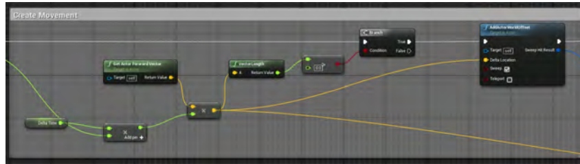
Figure 7.9: Create Movement Phase of Movement. This picture shows the Blueprint that handles how the player controller’s direction and speed are used to create movement.
