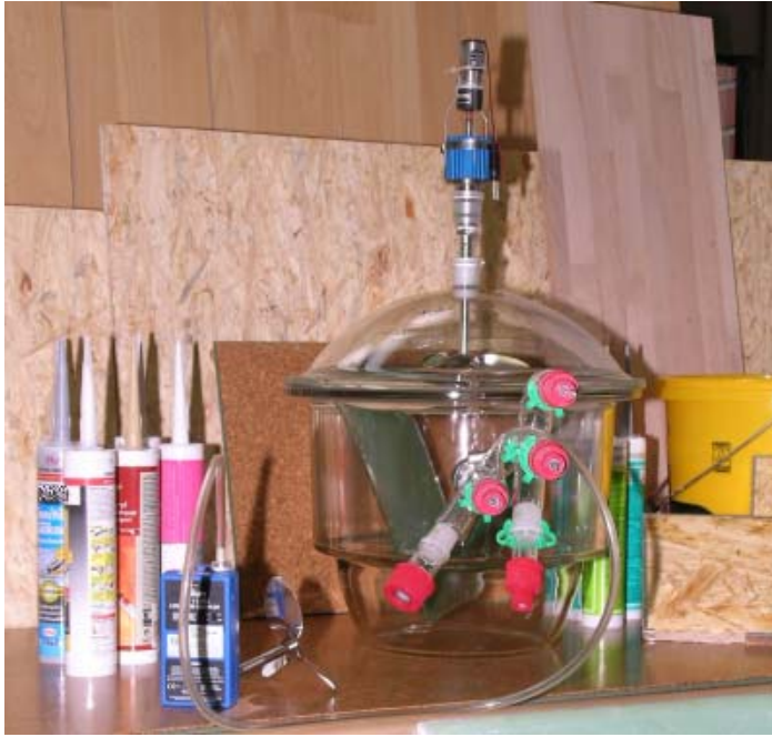
Figure 5-1: Building products and their emission tests in a 23-litre chamber
