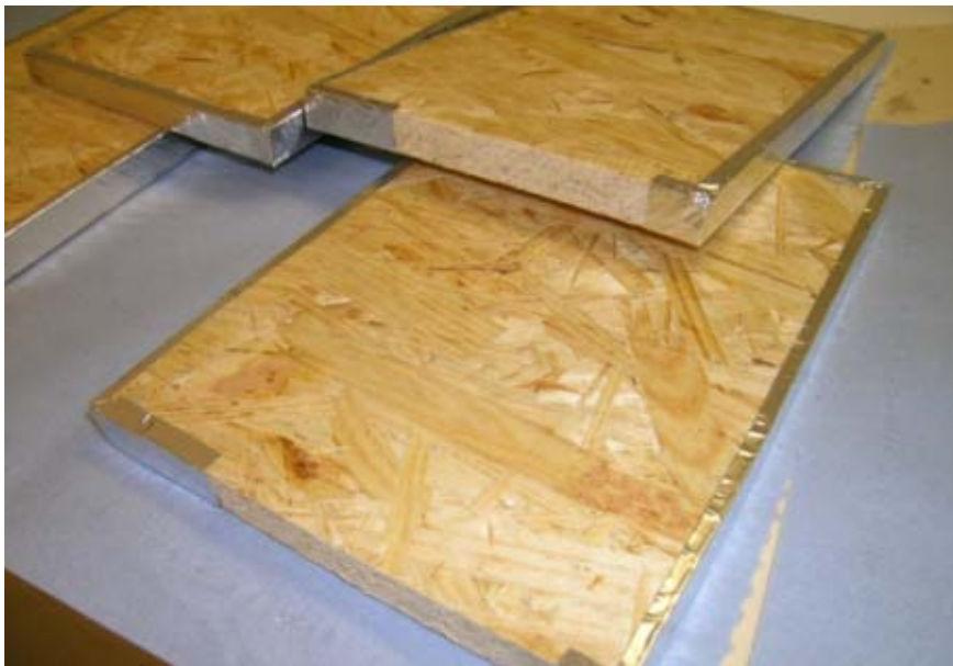
Figure 3-3: OSB prepared for chamber tests
