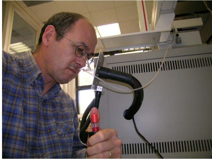
Figure 4-44: A panellist smells the eluate of the chromatograph (smell funnel and potentiometer)
