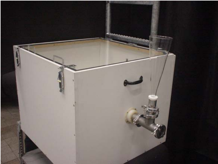
Fig. 10: Sampling and sample provision equipment AirProbe I
