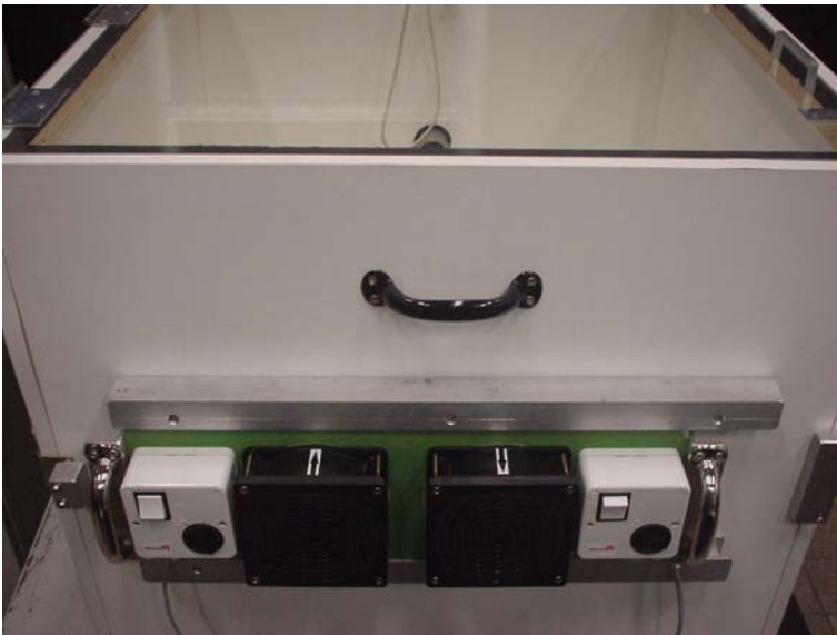
Fig. 11: View of the sampling device with the fans which can produce pressure or a vacuum in the casing
