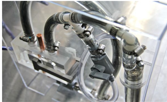
Figure 1.1: A modern MHD pump [5]. Photograph courtesy of Intellectual Ventures Laboratory.
