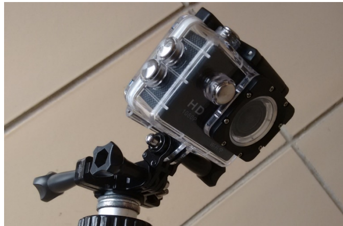
Figure 2: ANART Camera, Pole Mounted
