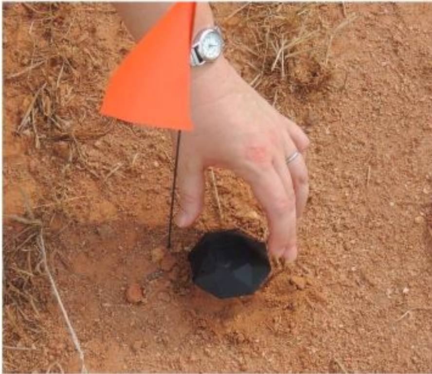
Figure 4. Example of a soil surface being scanned using the Nix™ Pro color sensor.
