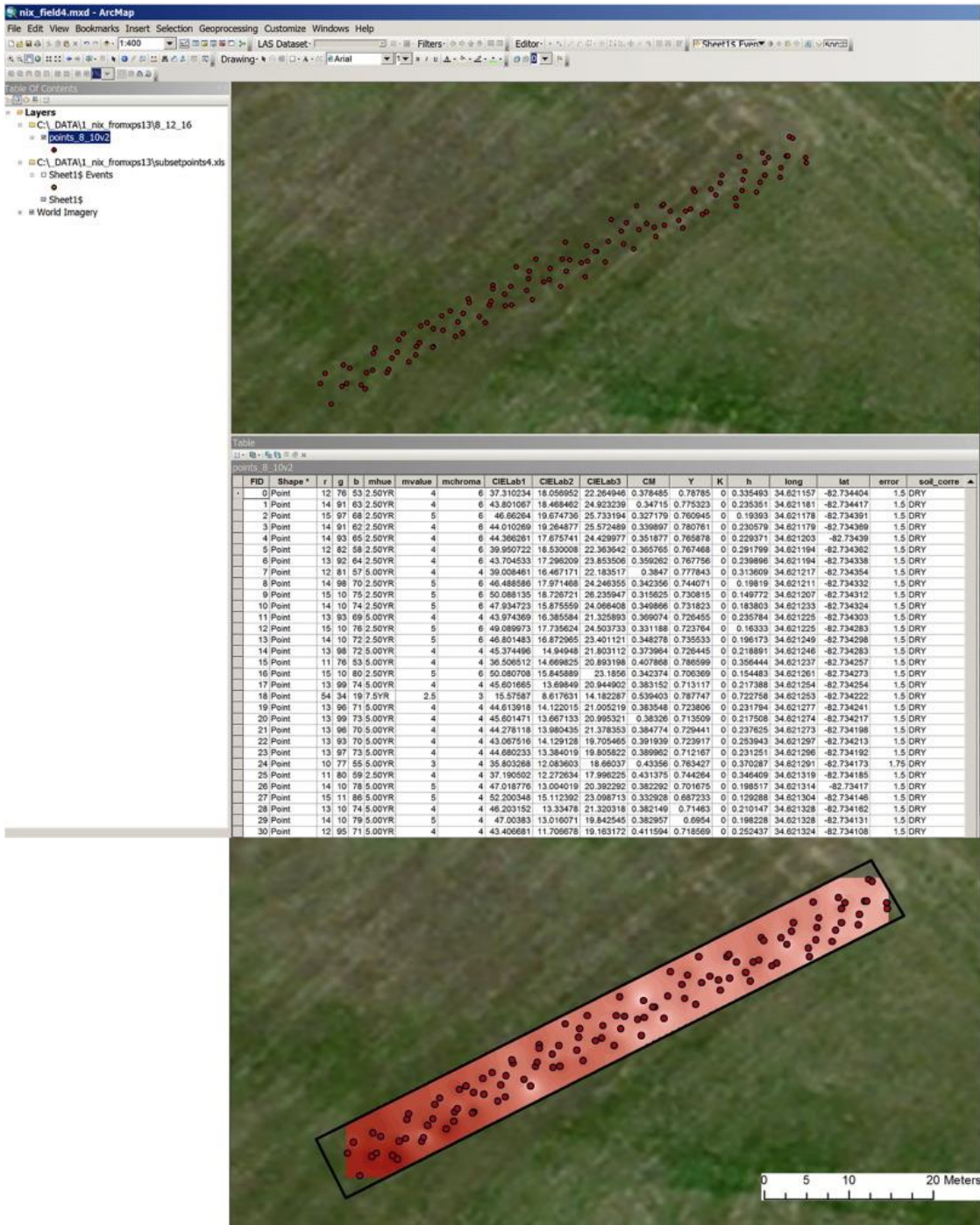
Figure 5. GIS layouts showing: scan locations (top), soil color attributes (middle), and interpolated a* (red) color values using Inverse Distance Weighting (bottom) for the Simpson Agricultural Experiment Station.
