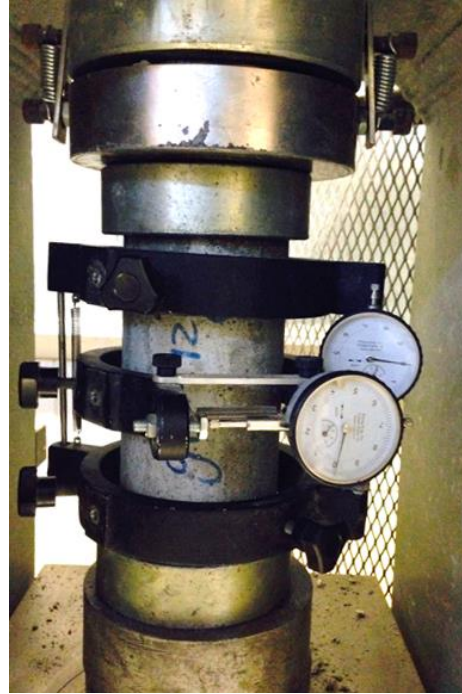
Figure 3-7. View of sample in compressometer cage to measure the MOE
