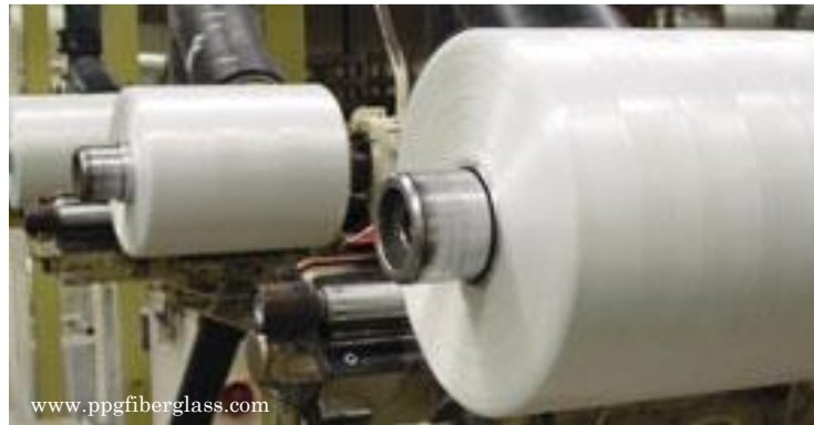
Figure 1-4. Production of glass fiber
