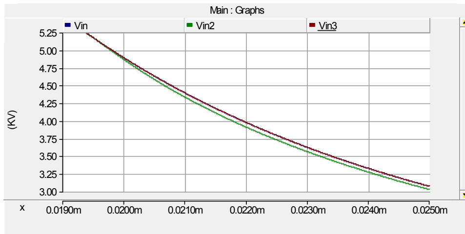
Figure 48: Pulse Response from Water-Tree
