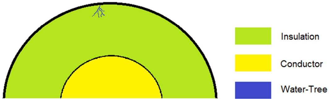
Figure 17: Water-Tree Branches in Insulation Layer
