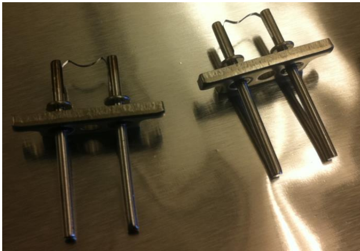
Figure 2.33 Sagging filament assemblies imaged after heating to high temperatures ( >1500 °C).
