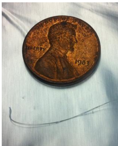
Figure 2.8 An image of a fiber prepared using the fiber formation method. Note: a fiber with a diameter of \sim 300 \mu\text{m} was imaged due to difficulties imaging thinner fibers without magnification.
