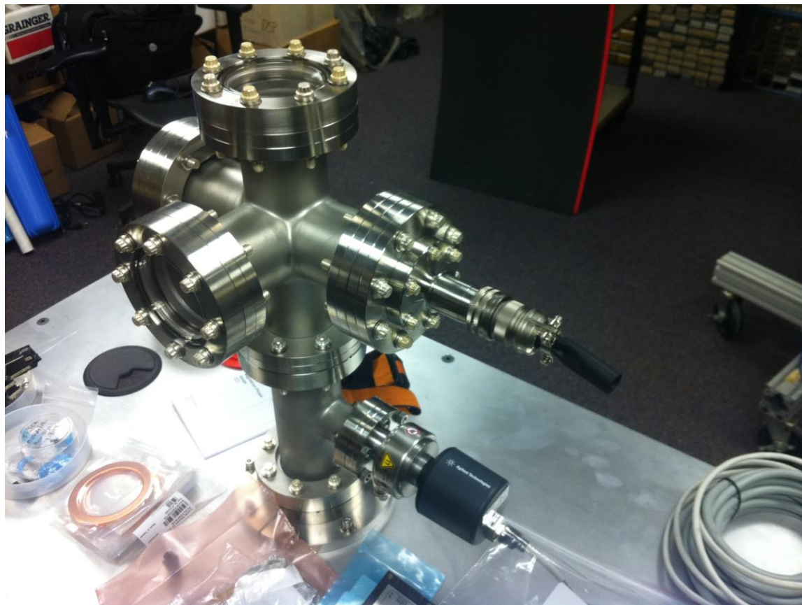
Figure 5.1 Thermal ion source created at Clemson University.
