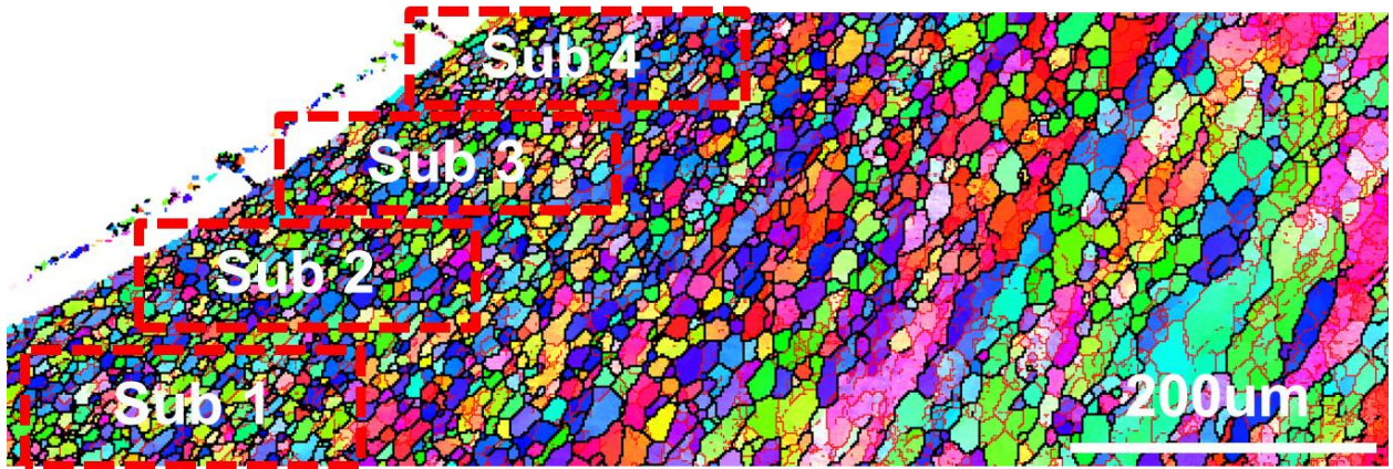
Figure 4.22 IPF image and subset selection near tube corner
