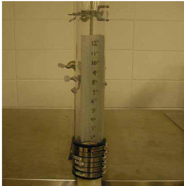
Figure 2.1 Falling head permeability apparatus for pervious concrete specimens (Schaefer et al, 2006)
