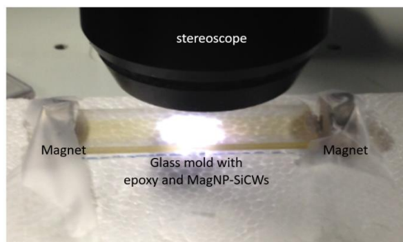
Figure 5.3: Experimental set-up for the observation of orientation of MagSiCWs at low concentration.
