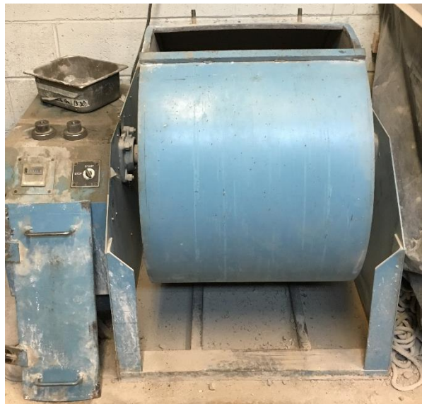
Figure 3.6- Los Angeles Abrasion Machine
