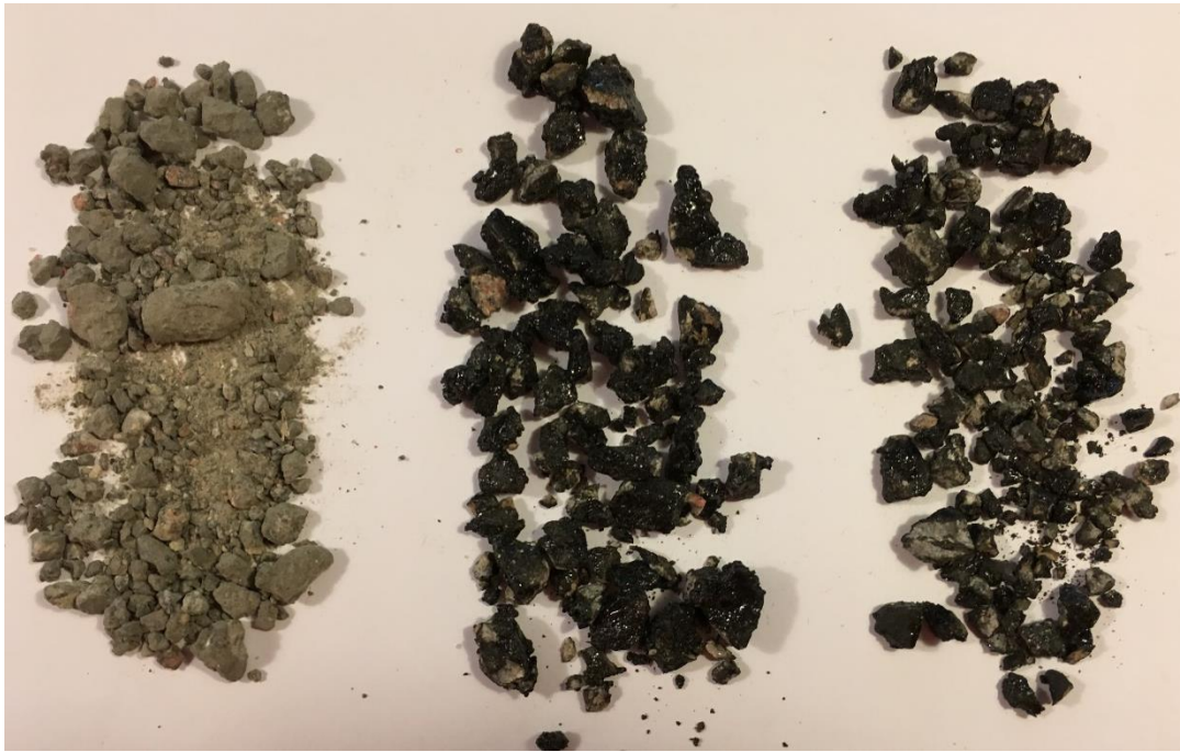
Figure 4.30- Dislodged Aggregate Particle from the Cantabro Test Method, Planetary Motion Abrasion Test Method, and Singular Motion Abrasion Test Method (Left to Right)
