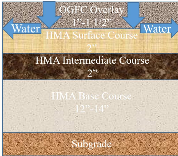
Figure 2.2- Typical OGFC Pavement Section
