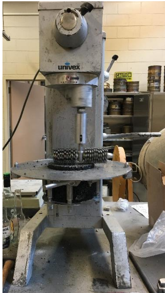
Figure 3.11- Planetary Motion Surface Abrasion Apparatus
