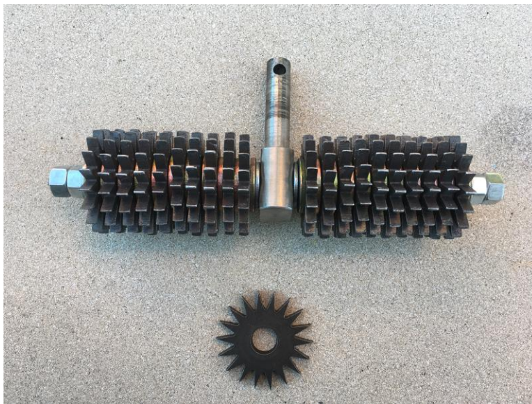
Figure 3.9- Triangle Rotating Cutter Head (Cutter Head B)
