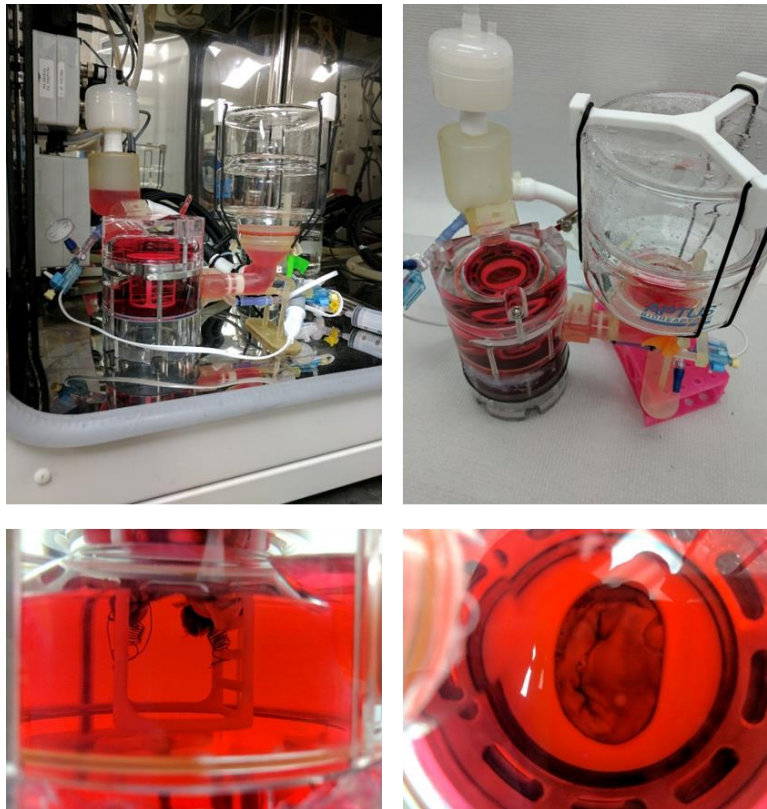
Figure 5.5: Assembly of the Mitral Valve Bioreactor. The overall structure of the mitral valve bioreactor is a modification of an aortic valve bioreactor. There are four chambers, an atrial chamber, ventricular chamber, air chamber, and an additional ventricular chamber. Also, present in this set-up is a large glass reservoir chamber, flow meter and two pressure transducers, which measure pressures in the atrial and ventricular chambers. In the center of the bioreactor is the mounted and seeded mitral valve construct. Pressure and flow is originated in the air chamber where air is pumped in, thus moving a silicone membrane. This membrane creates the flows and pressures desired for experimentation. Gas exchange is allowed through a sterile filter. The incubator in which this mitral valve bioreactor is placed controls all temperature, CO 2 levels, and humidity. Flow rate is also measured and can be adjusted using clamps.
