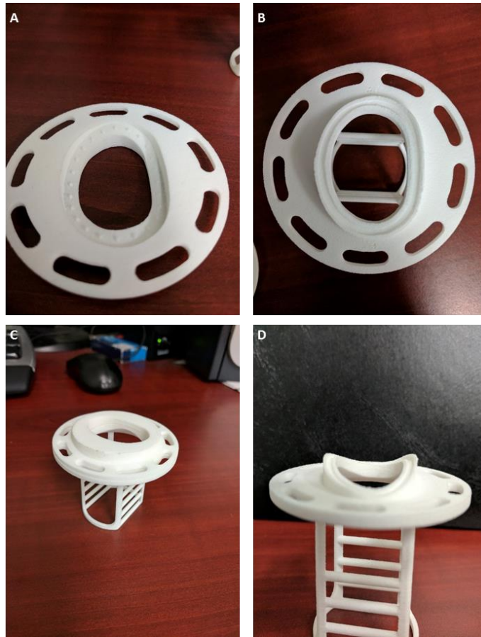
Figure 5.3: Development of the Mitral Valve Mount for Bioreactor Testing. A mounting ring was developed for the mitral valve as a modification to the already existing aortic valve bioreactor. The natural shape of the annulus was incorporated in this design to provide optimal force distribution throughout the valve during in vitro bioreactor testing. Also included were bars used to attach springs to the papillary muscles. This spring system allows for coaptation of the mitral valve at physiological pressures, while also providing proper tensile forces on the leaflets. This tension is also important for proper force applications in the chordae as well.
