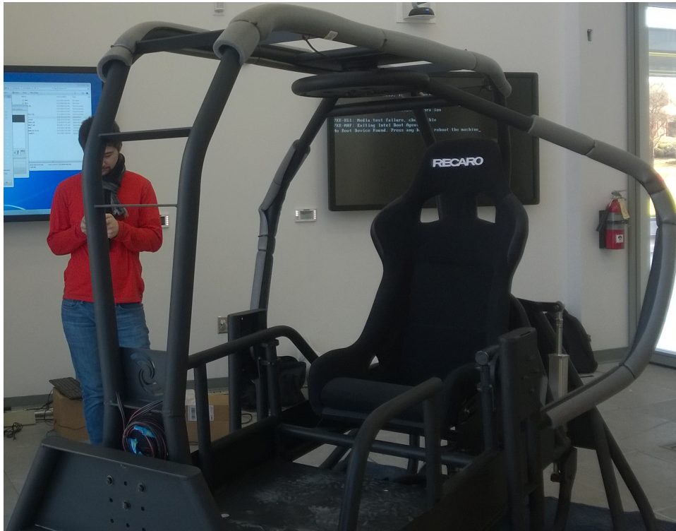
Figure 1.1: Physical rig responsible for providing haptic feedback
