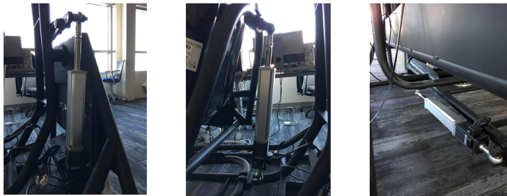
Figure 1.2: Stepper motors on the physical rig, Roll, Pitch and Yaw (Left- Right)
