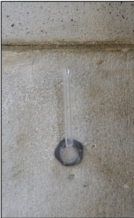
Figure 4.20: RILEM permeability testing of marble (Photograph by author).
